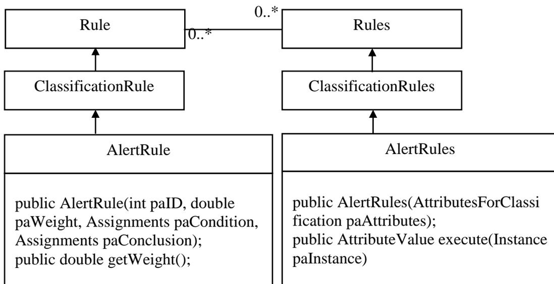
**Figure 3: Class diagram for alert rules.**
